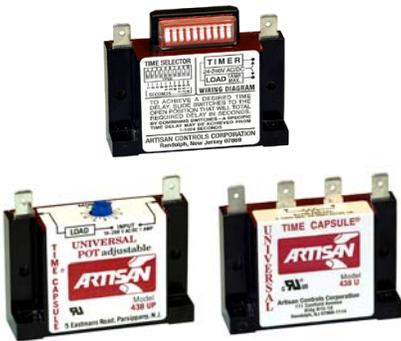
**Delay-On-Make:** (On-delay, delay-on-operate, delay-on-pickup, delay-on-energize): The timing period starts upon the application of the operating voltage, control voltage, or the closure of a separate initiate switch. After the timing period expires, the load is energized. Delay-on-make models are available in the Time Capsule®, 2" x 2", and plug-in case styles.
